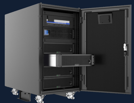
Three-phase 30-40 kVA UPS with 4 x 100Ah battery modules and 40 kVA PDM
