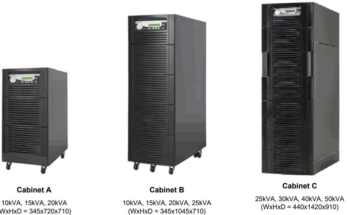
Figure 2.1 Kohler PW 5000/TP Cabinet details
